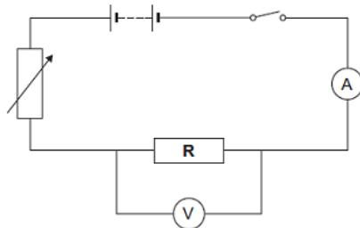
A resistor is a component that is used in an electric circuit. Describe how a student would use the circuit to take the readings necessary to determine the resistance of resistor R. (6)
